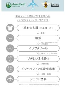
The project is to produce isobutanol by utilizing innovative biorefinery technology RITE Bioprocess<sup>®</sup>, which has been commercialized by GEI, from recycled cotton
